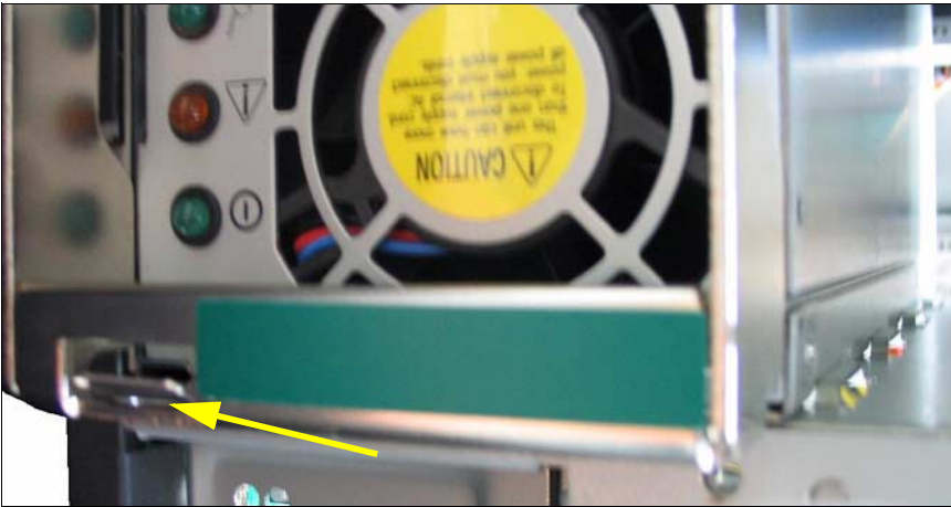
Figure 36: Locking the power supply module
